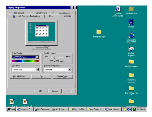
Move your mouse pointer over the bar under the words "screen area" click the left button, hold it down and move it left or right. When set click ok button. The higher the numbers the smaller the screen icons become.
